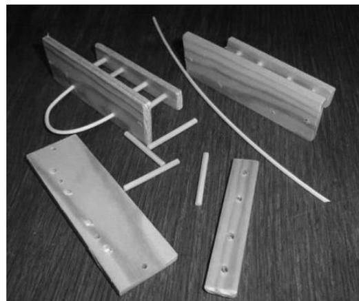
Fig 5, shows an assembled seat and the components that are required to make the seat. Once the seat is assembled it can be installed into the Coracle frame.
