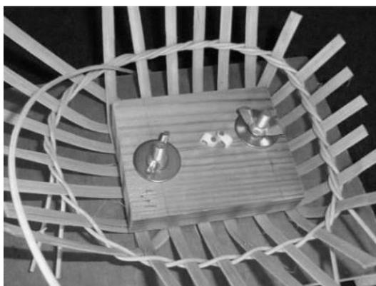
Fig 3, illustrates the frame being drawn up into a shape that is starting to look bowl shaped. The frame is held in place on the jig by clamping and this also helps create the flat bottom of the boat for which the Teifi Coracle is also renown.
