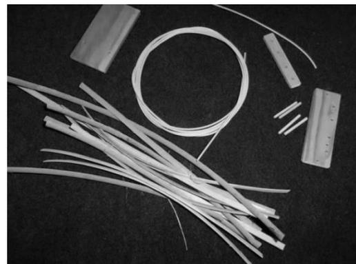
Once the raw materials are grouped together for the model, the soaking of the cane can be done to make the cane more pliable for weaving into the frame. The flat cane will be woven to construct the coracle hull/ body framework, and the smaller round cane will be woven in, to make the gunwale or rim of the boat.
